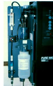
Orion's sodium monitor has been a star performer, the most populated so far in the power generation stations. My surveys show it represents over 60% of the total units installed.. Old by today's technology rules, it is a straight forward design that still meets the application need. When main-
